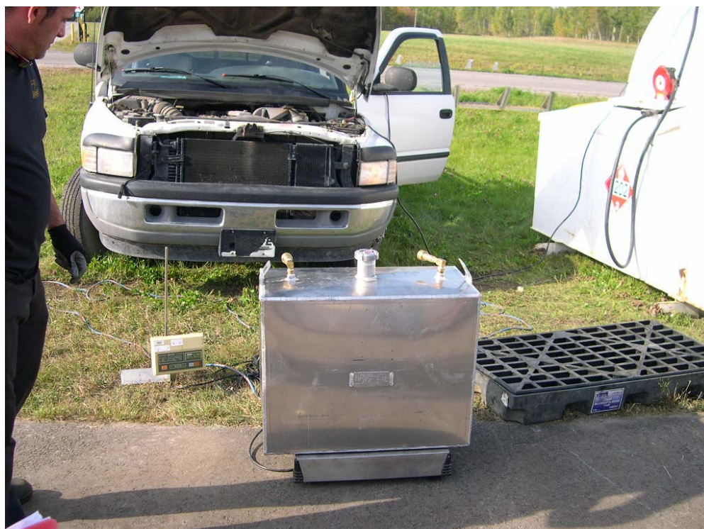
Figure 3. Temporary tank installation and weighing.
